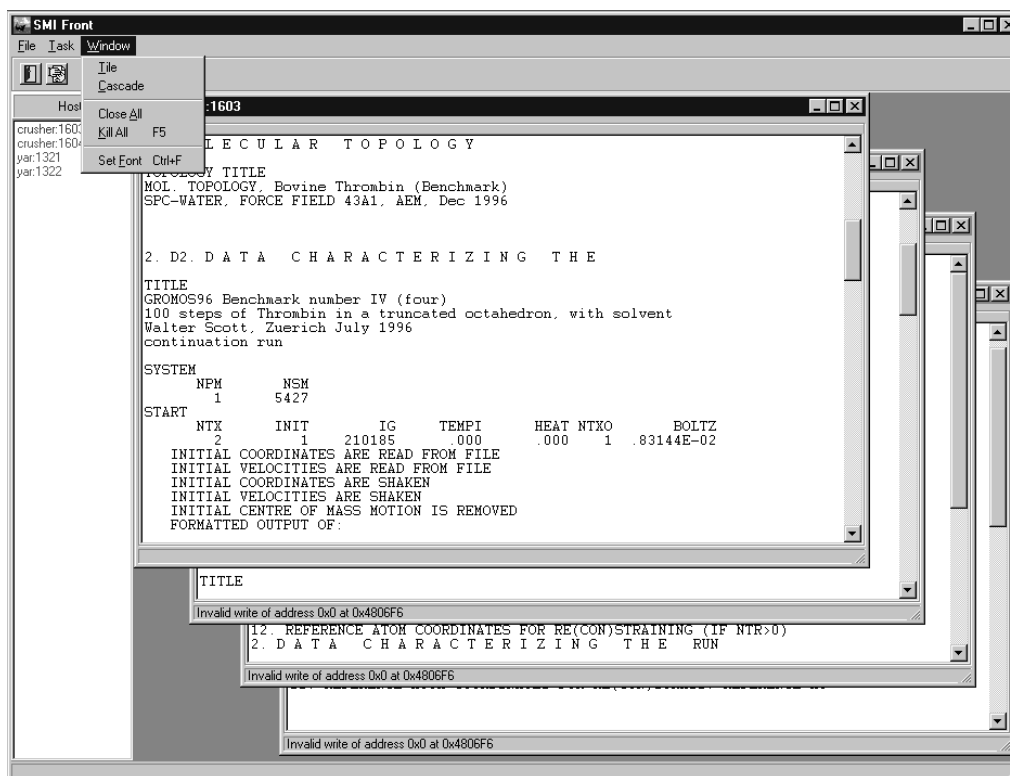
Figure 2: Screen-shot of SMI's window-based front-end. The output of a GROMOS96 run with 4 processes is redirected to the front-end on the user's machine.
