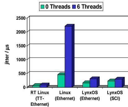
Figure 9. Jitter of the high-priority thread on various architectures
