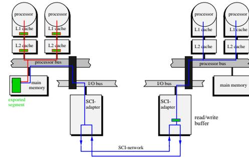
Figure 8. The system architecture of a SCI-Cluster
