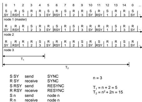
**Figure 5. Subdivision of time slots in example for three nodes**
