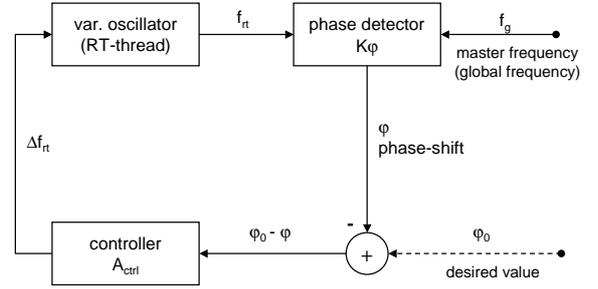
Figure 2. Structure of a PLL system
