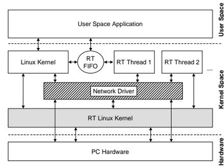
Figure 1. Parallel access to the time-triggered Ethernet driver
