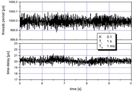
**Figure 7. Disturbance reaction of the control loop**
