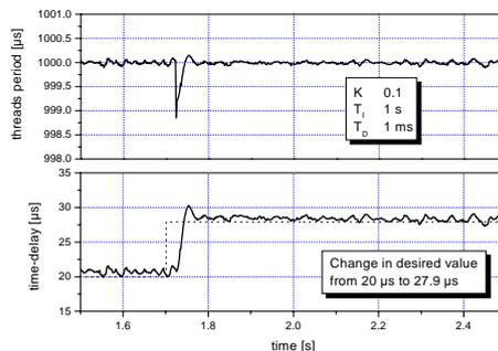
**Figure 6. Reference reaction of the control loop**
