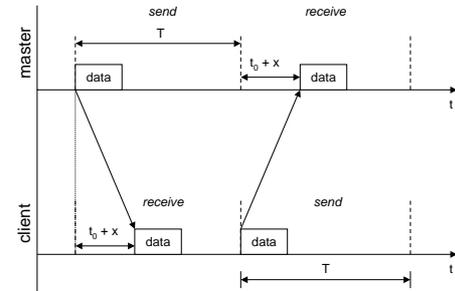
**Figure 4. Network timing after synchronization**
