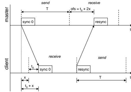
**Figure 3. Measurement of the propagation delay by a sync/resync-operation**
